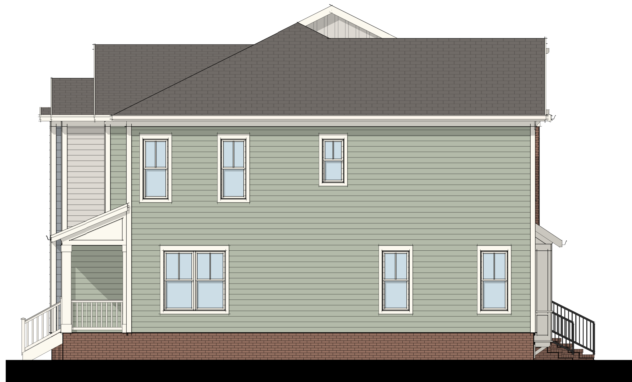
Townhouse (4-Unit) - Typical Side Elevation 3 3/16" = 1'-0"
