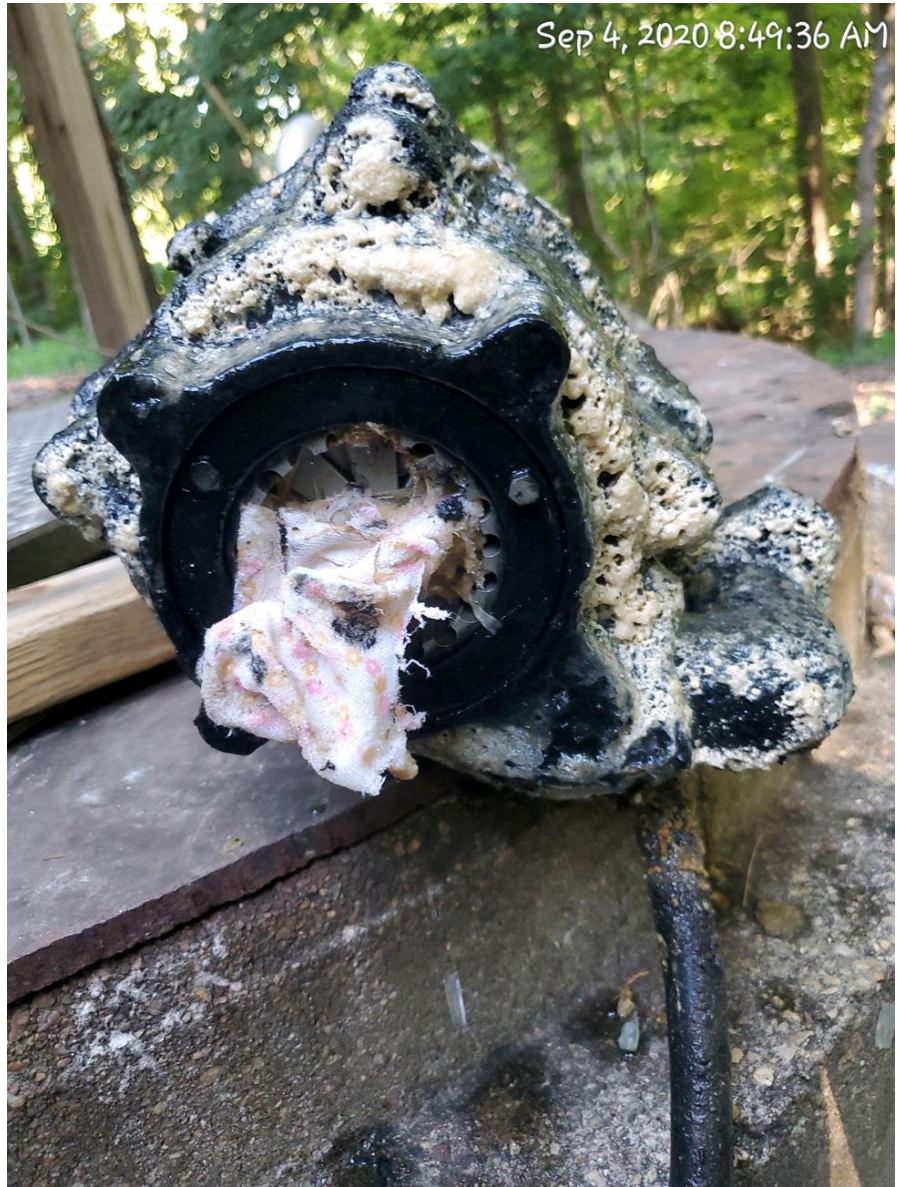
Oakdale Clogged Pump with Rags. 1Timbers PS Wet Well - Note corrosion.
