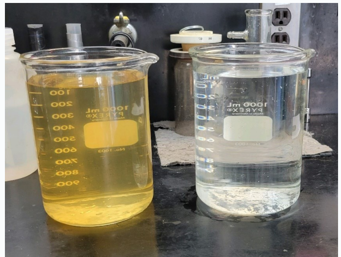
Staff at the Water Treatment Plant take raw water from the Eno River (left) and process it into finished water (right) that’s ready to send to your tap.
