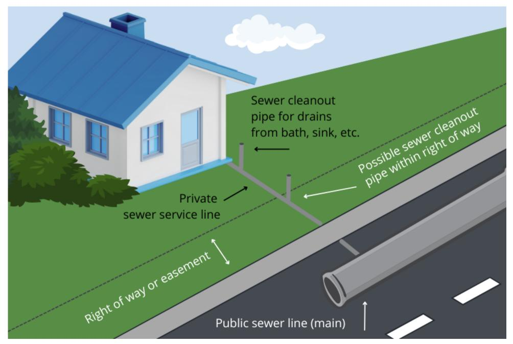
Lateral sewer service lines connect a home's sewer plumbing to the public sewer main. The town maintains the portion of the service line between the sewer main and the sewer cleanout pipe located at the edge of the road right of way.
