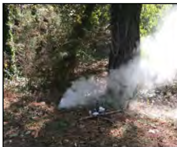
Figure 4: Smoke Escaping from Missing Cleanout Cap
